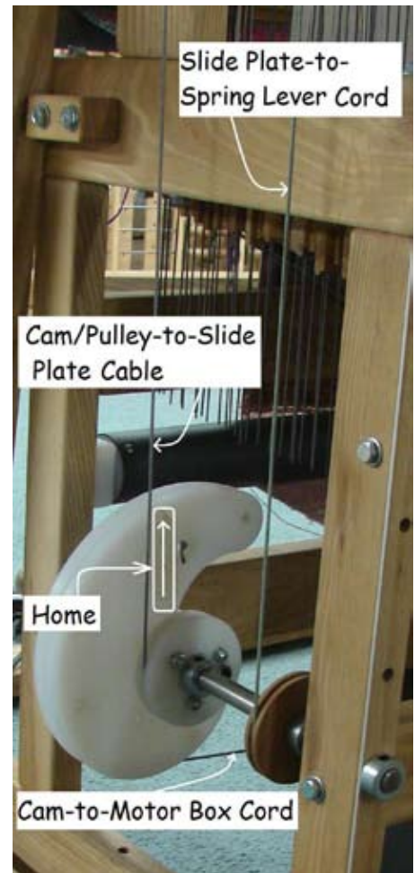
FIGURE 5-E: CABLE AND CORD INSTALLATION AND HOME POSITION
